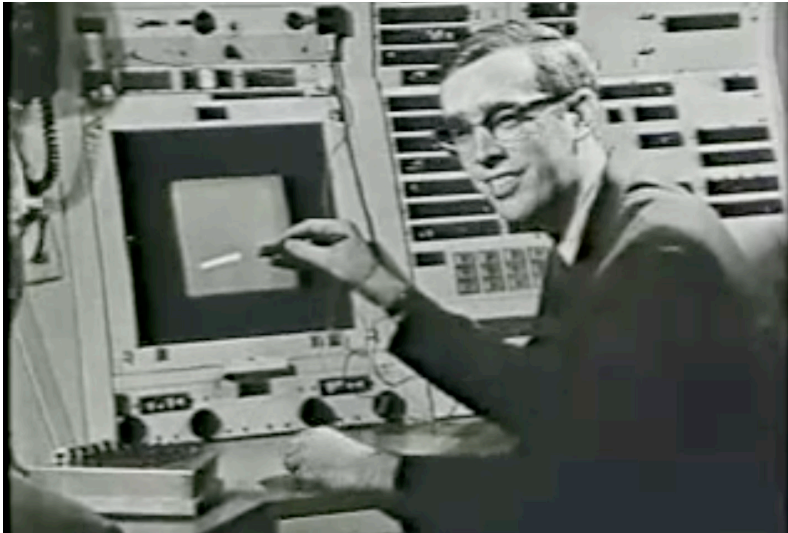
Figure 1: In a frame from the Lincoln Laboratory (1964) documentary, Timothy Johnson draws a line with Sketchpad's light-pen.
