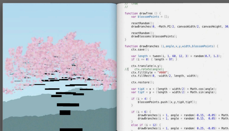
Figure 61: Bret Victor's (2012) IDE from Inventing on Principle . Since the programming environment is interactive, the code and the image are always in sync. As shown in the three frames, changes to the code also immediately change the image produced by the code – without the designer manually activating the Edit-Compile-Run loop to see them.
